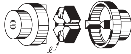
(b) Modified Spider Coupling ( \ell - lip providing bulging space for the rubber element)
